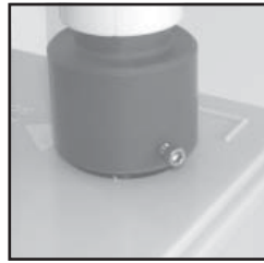
Back out lock screws
