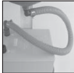
Transfer Tube Installed
